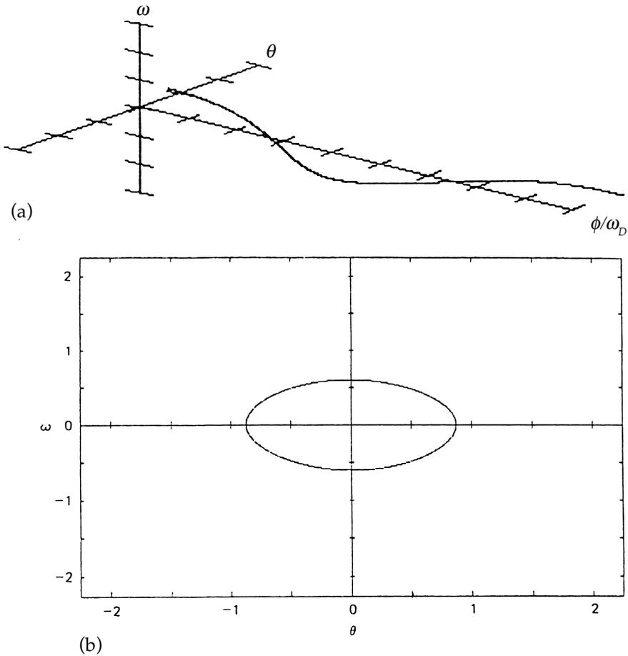
Fig. 3. Geometrical representations of the dynamics of a simple oscillating pendulum. In (a) the angle, angular velocity, and time form a triplet of axes for the motion. The back and forth motion is represented in this new “space” by a spiral. In (b) the time dimension is suppressed and the motion in the two dimensional space of angle and angular velocity forms an ellipse.
