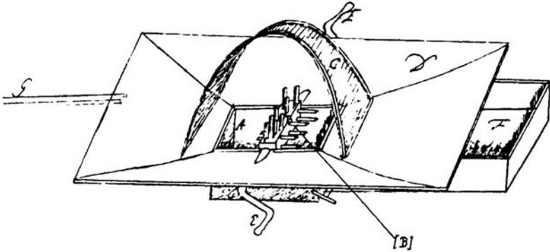
Fig. 4. Beam cd is driven back and forth constantly by a pneumatic machine or windmill. It turns the cylinders or axes e, e, e, e, and they raise the hollow vessels f, f, f, f, f and lower them on the other side,
