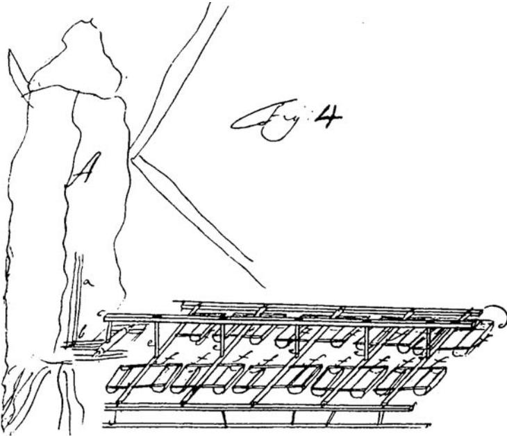
where they refill with water. When raised on the other side they spill the water out again, and so continually. It is thought that thus the water, by being continually taken out and poured back, is dissipated as vapor, and that what remains will be rendered suitable for evaporation.
