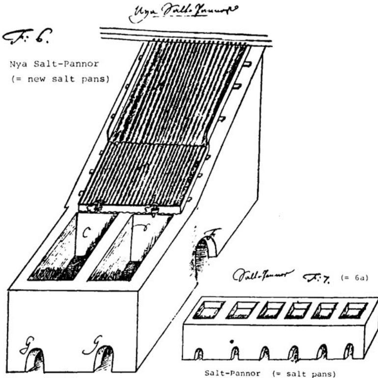
Iron sheets are placed on a slope, A, [corrugated] with small channels in them. The water flows down these sheets into the lower vessels
