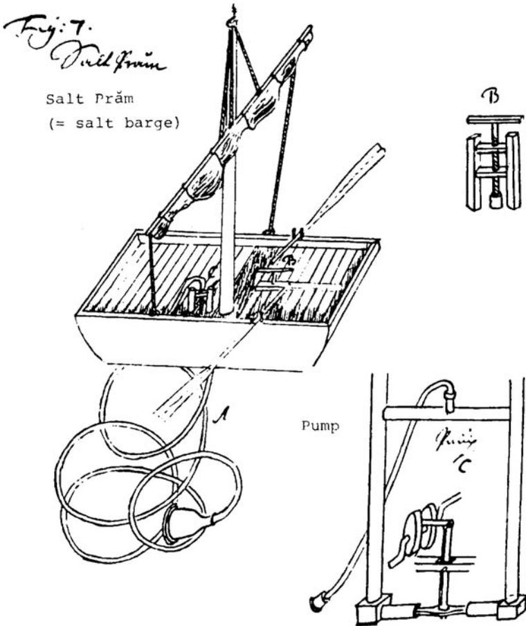
bottom than near the surface. A leather hose [A] is thrown into the sea, with a weight on the end which pulls it down. When it has been let down all the way, they open a hole in the bottom of the boat with
