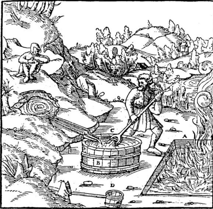
Trench A. Vessel into which salt water is diverted B. Spoon C. Jar attached to a pole D.
